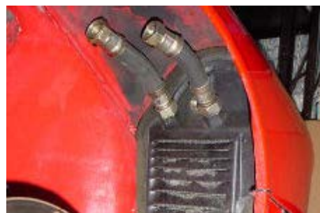
Front fender with cooler and flex-hoses installed
