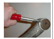
3 – Position the split bushing removal tool so that the small "teeth" are positioned at the parting line between the two bushing halves. Gently tighten (25 inch lbs) the bolt on the split bushing removal tool to separate the tool jaws and engage the bushing half.
