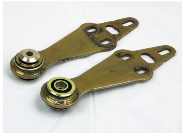
Monoball cartridge installed in original spring plates
