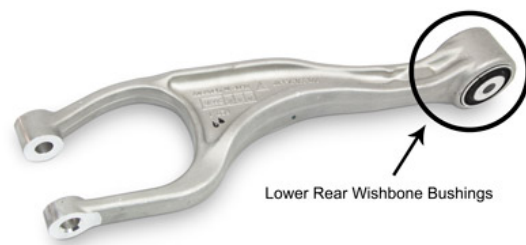
Monoball cartridge installs into the bushing location
