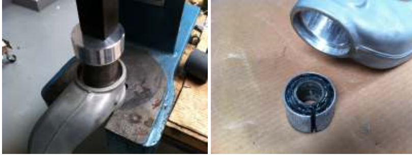
Press out center bushing
