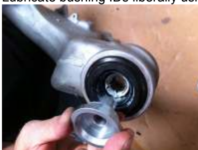
Press in pivot assemblies
