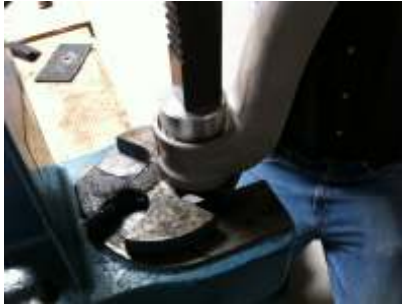
Press in center bushing using provided tool
