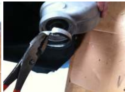
Chisel metal casing to separate from trailing arm, pull out metal casing with pliers
