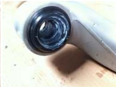
Lubricate bushing IDs liberally using provided grease
