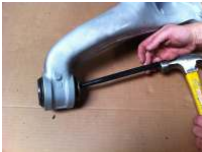
Drive out center metal pivots
