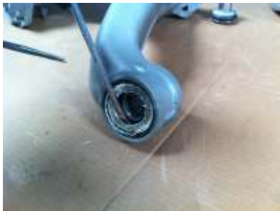
Pry off thrust washers, cut slit in metal casing of side seal
