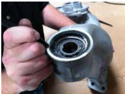
Chisel metal casing to separate from trailing arm, pull out metal casing with pliers
