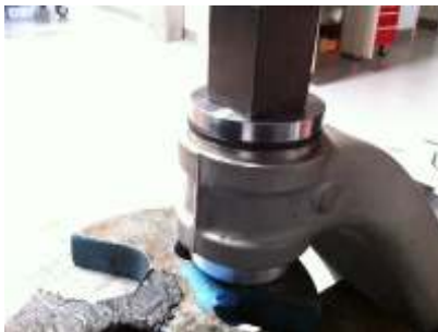
Press in side bushings using provided tool
