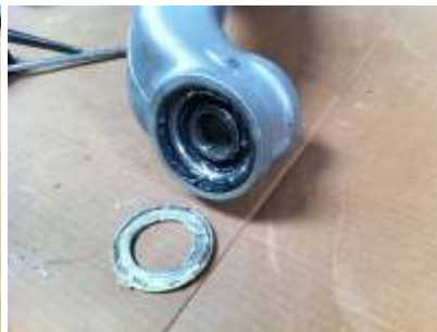
Pry off thrust washers, cut slit in metal casing of side seal
