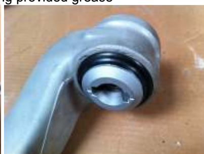
Lubricate bushing IDs liberally using provided grease
