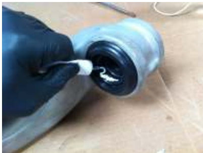
Lubricate bushing IDs liberally using provided grease
