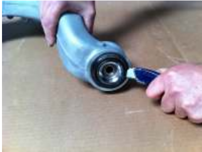
Cut around rubber seal
