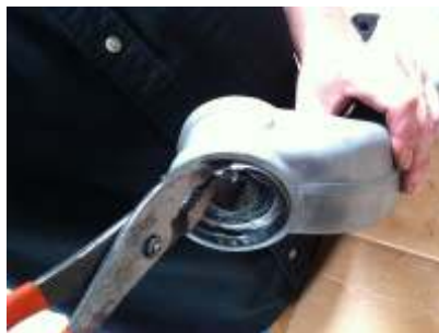
Chisel metal casing to separate from trailing arm, pull out metal casing with pliers
