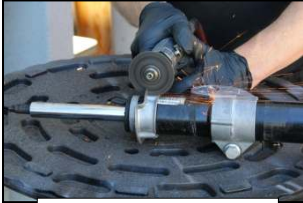
Photo 1: Cutting lower spring perch
