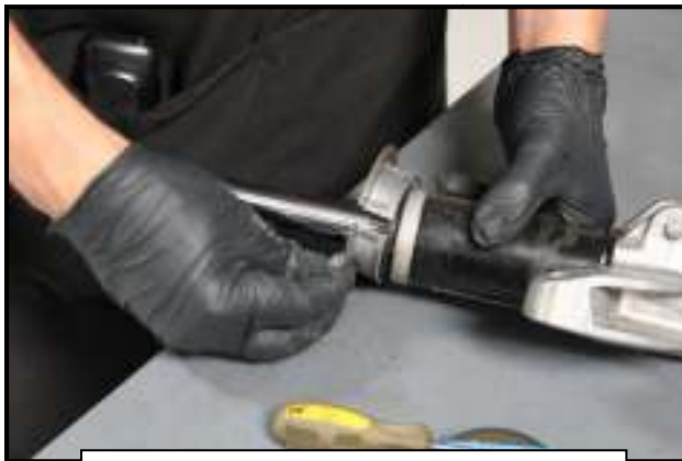
Photo 2: Removing Lower Spring Perch from Strut Body
