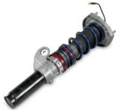
Photo 4: Assembled Coilover Strut
