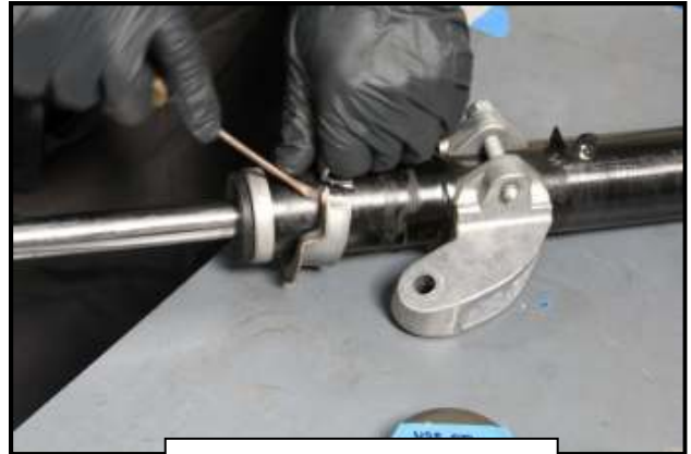
Photo 3: Prying Apart Lower Spring Perch
